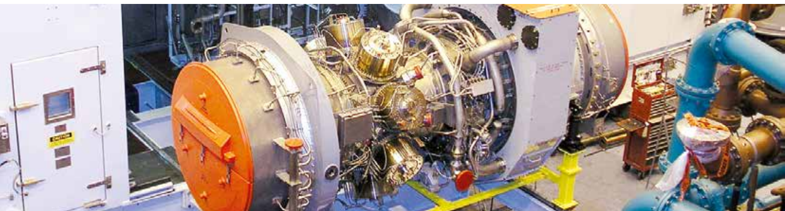
The Industrial Trent 60 MD - the best mechanical drive for LNG refrigerant compression
